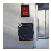
2. Plug the gun into the cable. Turn the gun "on". Push the trigger all the way forward to activate, this is a safety feature. Now, gently and slowly, pull the trigger back and walk next to the board. As the trigger is pulled, it will accelerate.
